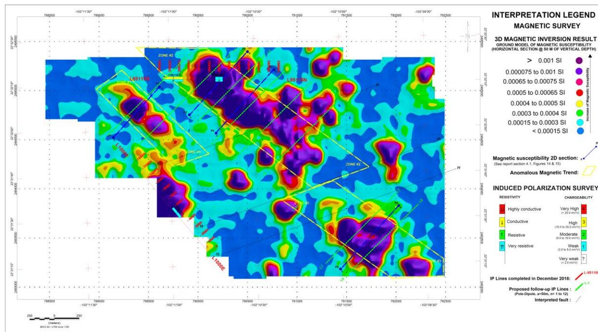
**Ground magnetic survey anomaly with proposed IP lines perpendicular (green), Donovan 2, January 2020**
