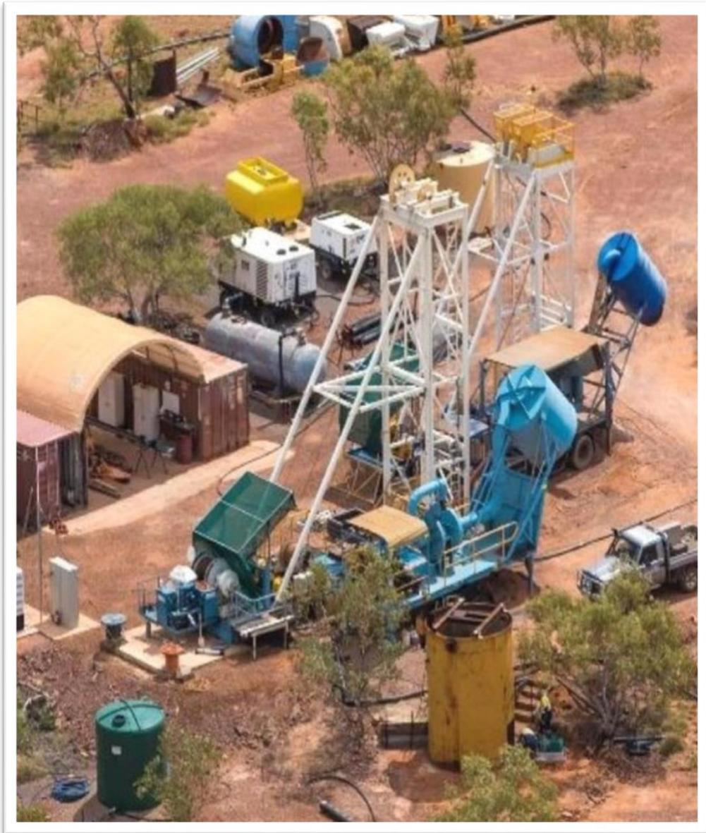
**Figure 2: Headframes, gensets, compressor, workshop on site in NT prior to dismantling for transport to Elizabeth Hill**
