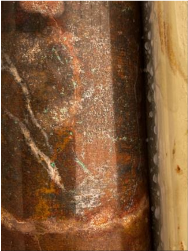
Native silver with associated copper (green) in drill core, drillhole EHDD003, 16.5m depth, Elizabeth Hill, September 2021
